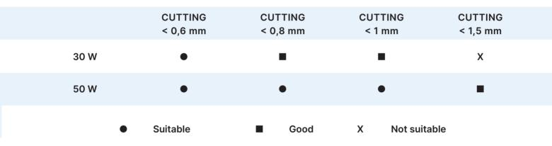
Except for titanium and steel, where cutting is only possible for simple geometries with a maximum thickness of 0.4 mm.
